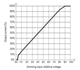
Applying additive 10V PWM signal (frequency range 1KHz ~ 3KHz):
