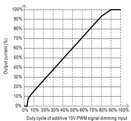
Note: 1.Min.dimming level is about 8% and the output current is not defined when 0% < lout < 8%.
