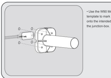
• Use the W90 Mounting Bracket as a template to mark the screw holes location onto the intended surface covering over the junction-box.
