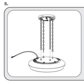
• Hang the fixture from the four chains by inserting the spring loaded hooks through the round eyelet anchors located on top of the fixture.
