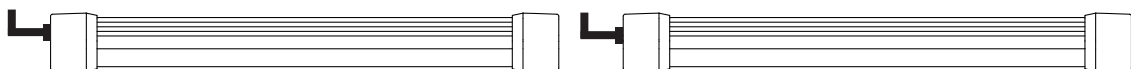
WP - Single Pre-Installed Cable Gland with cable wire on one side of each fixture for parallel connection
