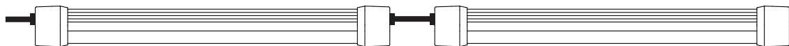
WS - Dual Pre-Installed Cable Glands with single cable wire on one side of each fixture for series connection
